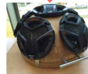
Students transformed wooden salad bowls from Ikea into omnidirectional audio speakers.
